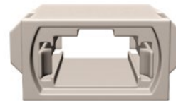
Adapter with TYPE B polarity shows two keyways on the same side. The connectors are connected 0° in relation to each other, both are in the same position. Gray in color.
