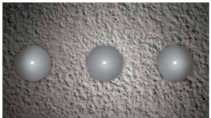
Core of a single-mode LC Connector.
